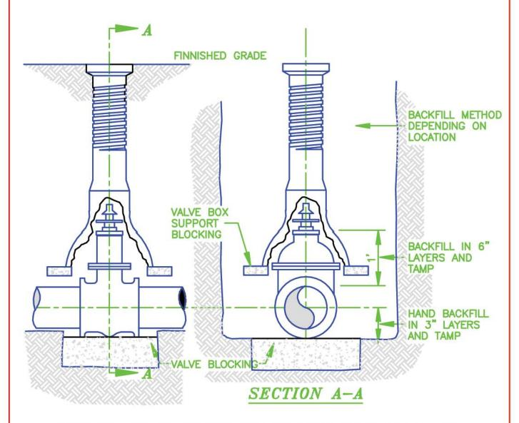
VALVE BOX SHALL BE CENTERED AND PLUMB OVER THE WRENCH NUT AND SHALL NOT TRANSMIT SHOCK WAVES OR STREES TO THE VALVE.
